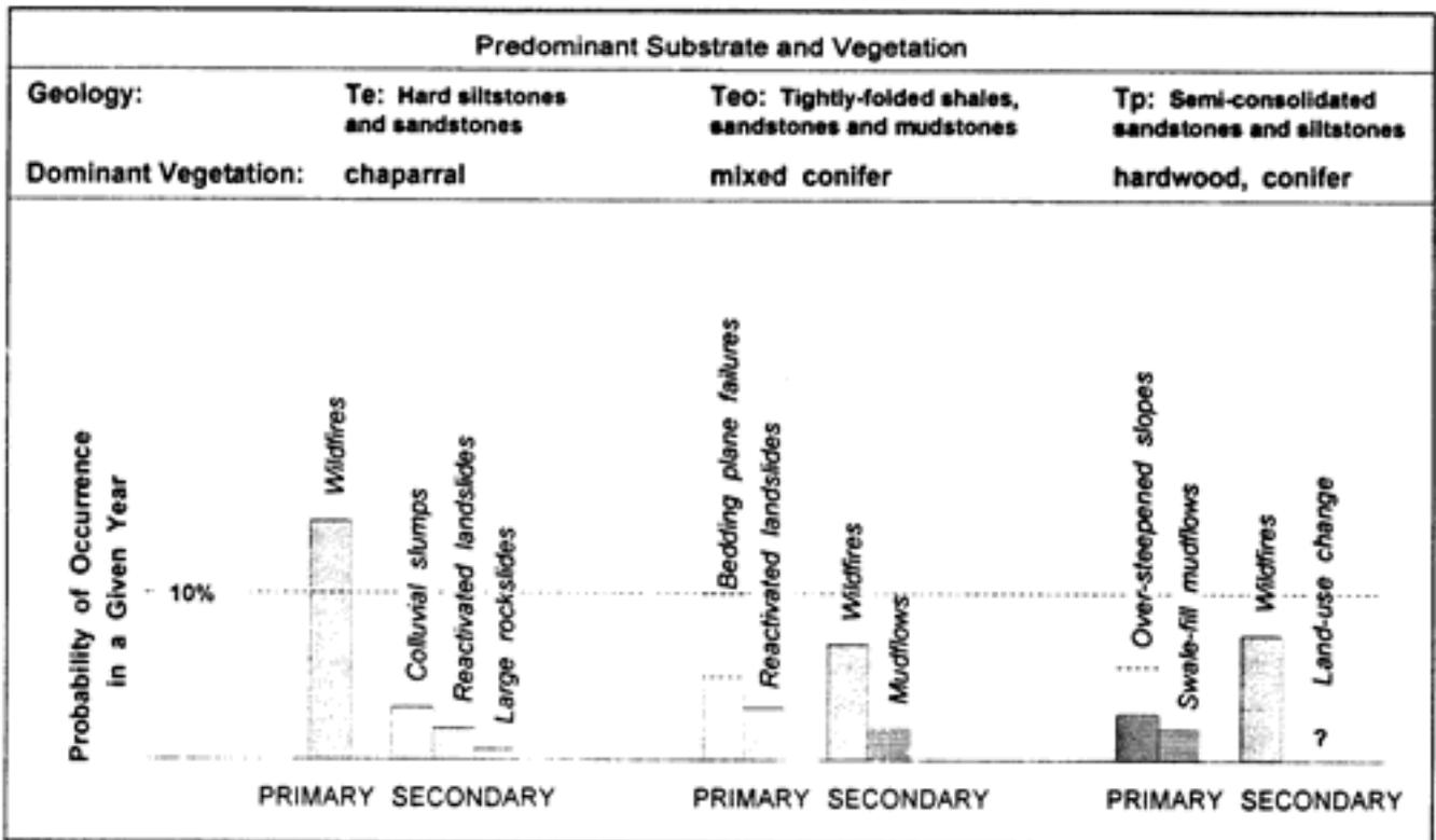
Figure 7. Estimated probability of significant sedimentation of steelhead habitat caused by episodic events, in three geologic/vegetative regimes, Corralitos Creek watershed. Probabilities based on estimated or observed frequencies and projected durations of bed sedimentation. Primary disturbances warrant site assessments by knowledgeable specialists and may merit temporary management measures. Secondary influences are more localized or less severe than primary. Source: Hecht and Woysner (1991).
