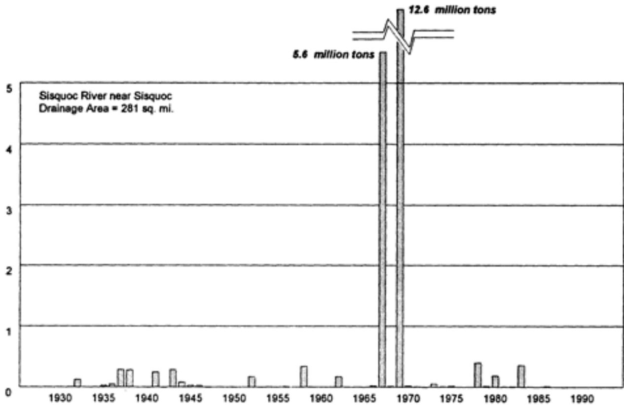
**Figure 3. Simulated long-term record of bedload sediment transport in an unregulated episodic stream-- the Sisquoc River, near Santa Maria, California. More than half of the bedload (coarse) sediment transported by the river during the 60 years was probably associated with two events -- the Wellman fire (1966), which burned approximately 35 percent of the watershed, and high-recurrence storms of January and February 1969. Source: Knudsen et al. (1992).**
