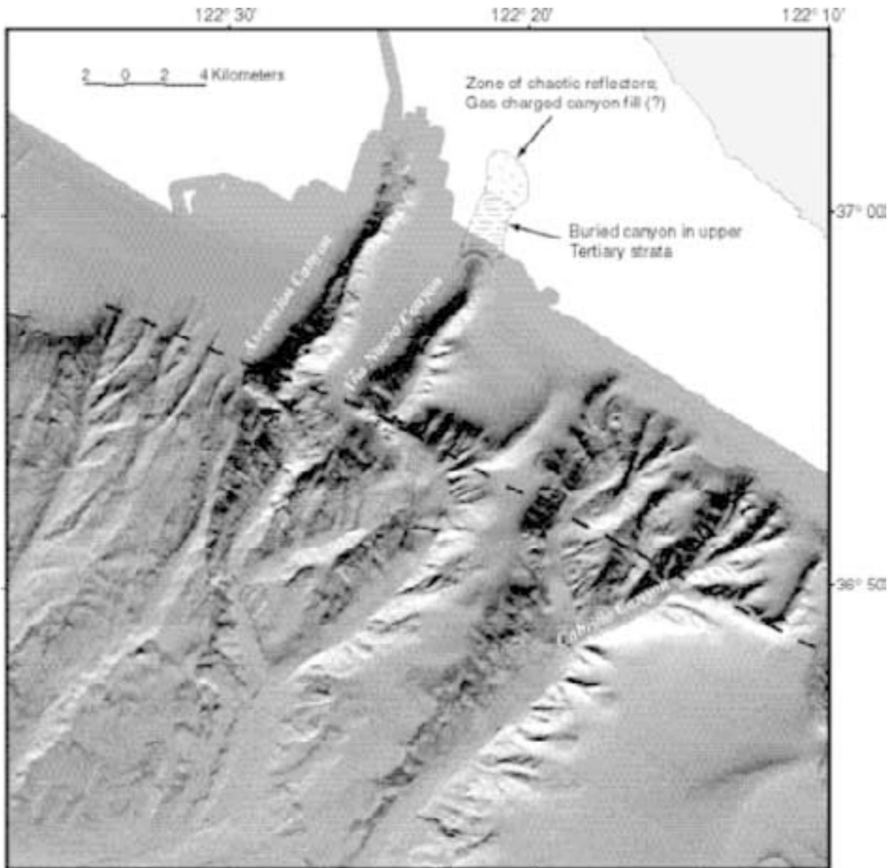
Figure 10. Shaded relief map of Ascension Canyon slope showing inferred gas induced canyon head collapse at Año Nuevo Canyon. Dashed line represents inferred structural lineament, possibly a fault or lithologic contact. Map constructed from MBARI EM300 multibeam bathymetry. Slashes and dashed symbols indicate the location of interpreted gas occurrences near the head of Año Nuevo Canyon by Mullins and Nagel (1982).
