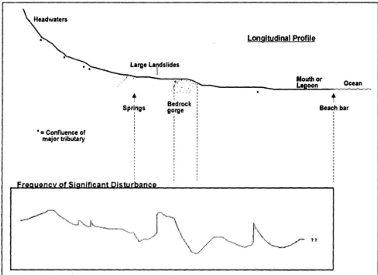
Figure 4. Schematic longitudinal variability in the frequency of episodic disturbance in a representative central California corridor. Reaches immediately downstream from channel confluences and other point sources of sediment are more susceptible to frequent disturbances; reaches with gorges or perennial springs tend to be more resilient to the same disturbances. Frequency diminishes from upstream to downstream, but relative severity or extent of disturbance does not.
