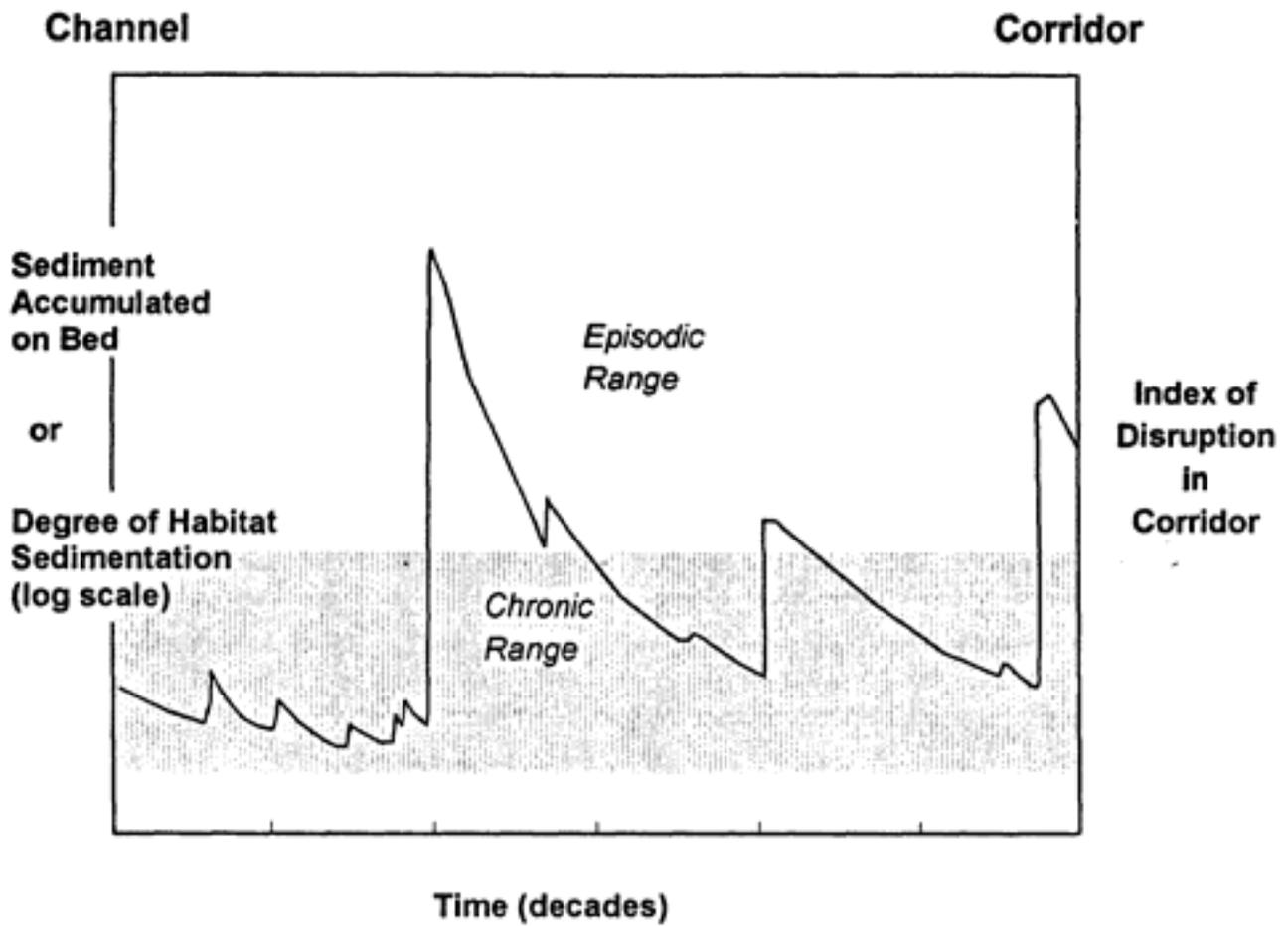
**Figure 1. Schematic representation of episodic variations in bed sedimentation and/or disturbance in riparian alluvial-scrub corridors of central or southern California streams.**
