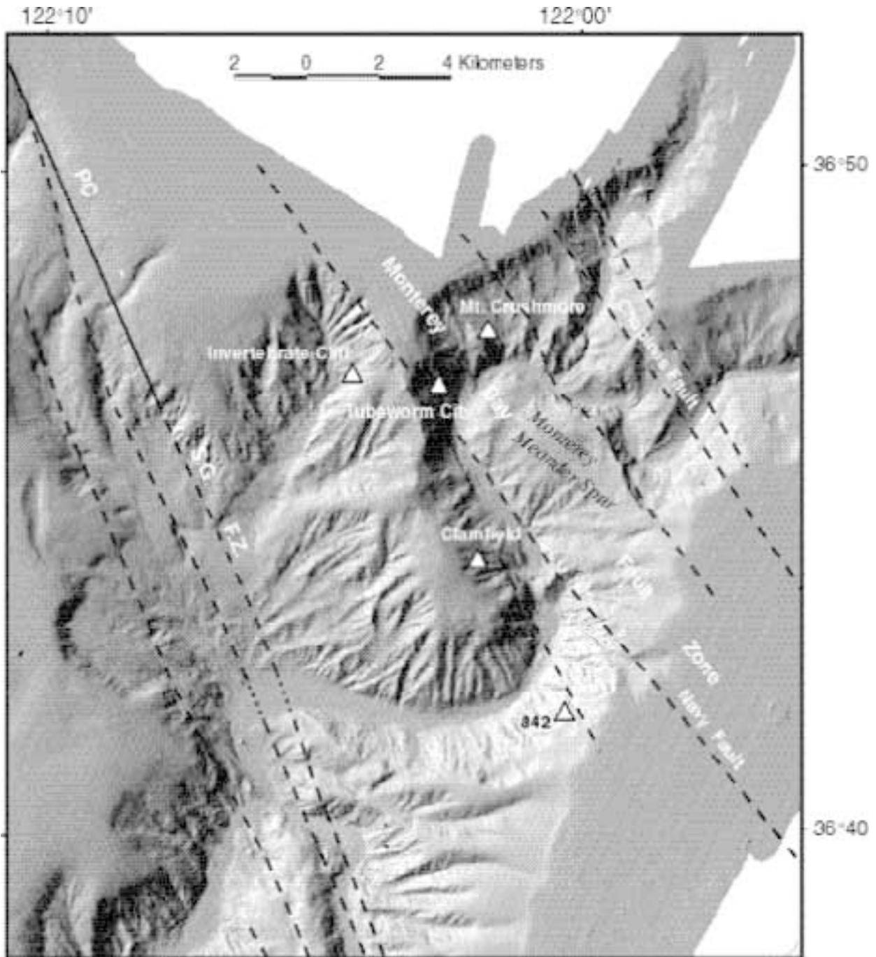
Figure 6. Shaded relief map of the Monterey meander and spur located within the middle part of Monterey Canyon. Seafloor morphology, faults, and active seep sites are shown and labeled. Map constructed from MBARI/USGS EM300 multibeam bathymetry.
