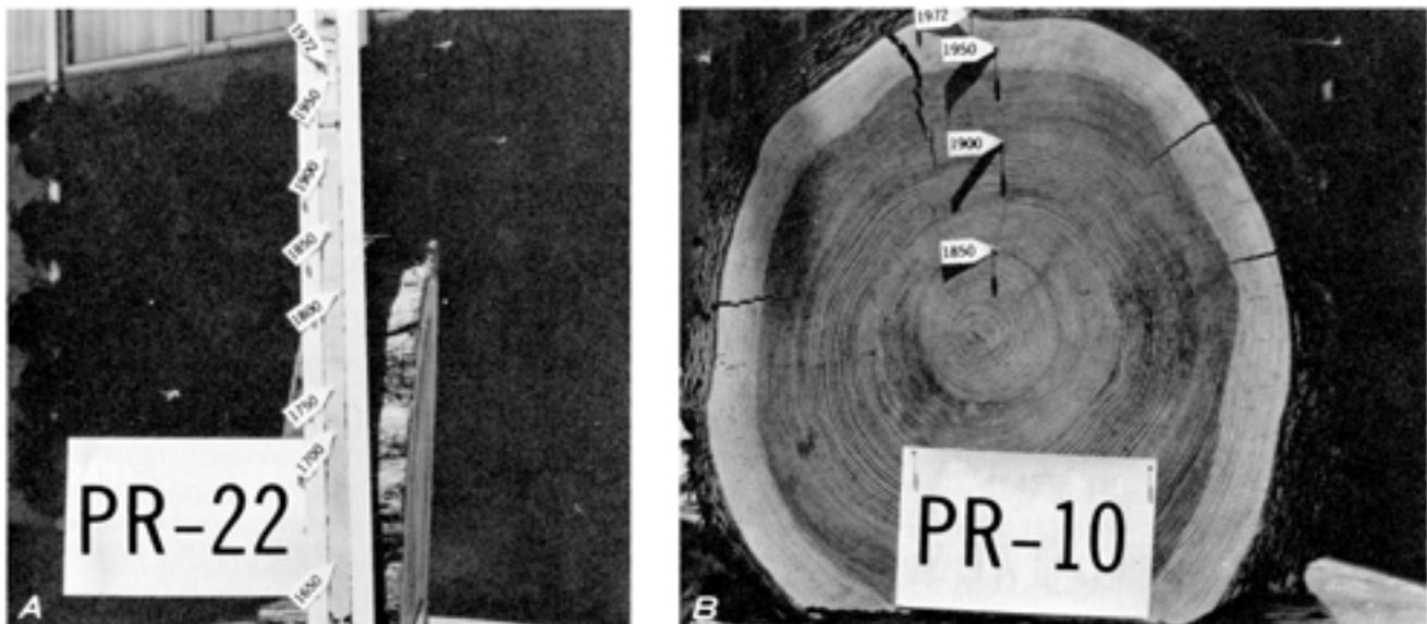
FIGURE 8.—Examples of core and slab samples prepared for annual-growth-ring studies. *A*, A part of the core taken from tree PR-22. The core was oriented for ring counting, bonded to the pregrooved mounting board, and sanded flush with the mount. *B*, A slab from fallen redwood PR-10. Note that the ring widths vary and that some of the rings are discontinuous. The cards are 5 by 8 in (139 by 200 mm).
